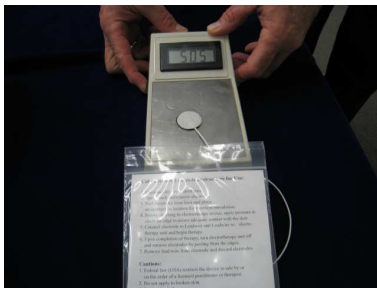
Columbia Scientific 600 Series electrode. Tested impedance of 505 \Omega
