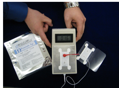
eSWALLOW USA electrode. Tested Impedance of 16 \Omega
